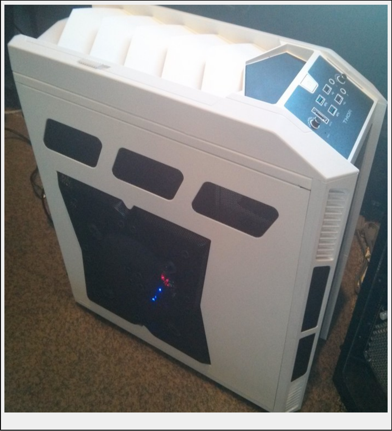
Fig 1.14 - GPU Mining Computer Exterior (3x GPU cards, 1050w power supply)
