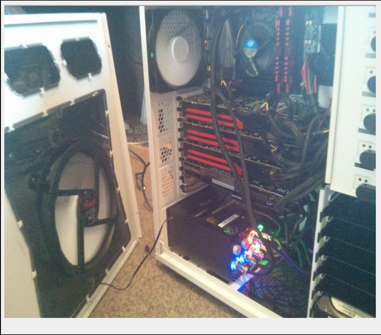
Fig 1.13 - GPU Mining Computer Interior (3x GPU cards, 1050w power supply)
